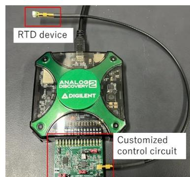
**Fig.2** The integrated RTD sensing system, which can be applied for the 3D imaging and precise thickness measurement by connecting to a laptop, as introduced in section (b).
