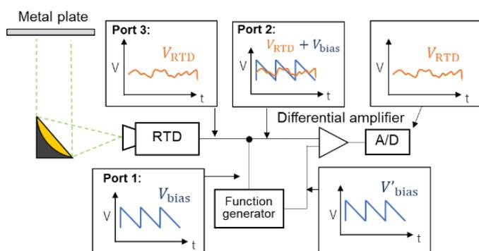
**Fig. 1** Concept the FMCW radar using an RTD transceiver. The RTD module was connected to Port 3 of a T-bunch, which was used to provide bias voltage  $V_{\text{bias}}$  to the RTD module at Port 1. Both voltage of the self-mixing signal  $V_{\text{RTD}}$  and  $V_{\text{bias}}$  were detected at Port 2. A differential amplifier was employed to extract  $V_{\text{bias}}$  using a synchronized channel  $V'_{\text{bias}}$  from a function generator.
