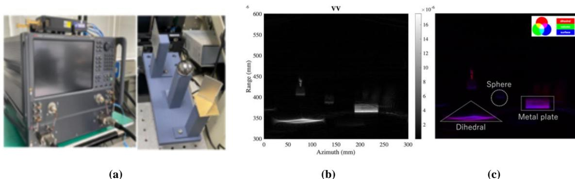
**Fig.4** THz imaging using VNA system; (a) experiment setup; (b) conventional imaging result; (c) target classification using polarimetric information.
