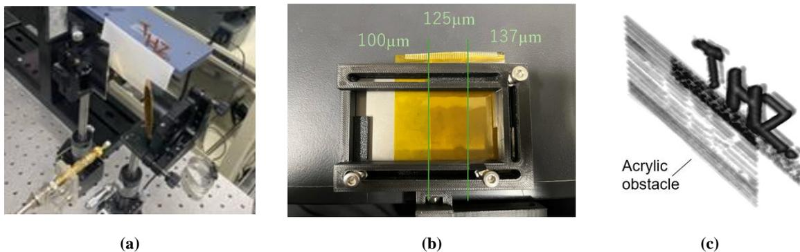
**Fig. 3** (a) Imaging/sensing configuration using the proposed system; (b) layer material model used for the thickness measurement; (c) 3D imaging result including an obstacle at the front. The target consists of three characters, “THZ” made using a 3D printer, with a width of 15 mm.
